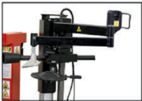
RP11-52PT230 Bead Press System ➤ Right side mount ➤ Mount head roller and press head ➤ Lifting disc
